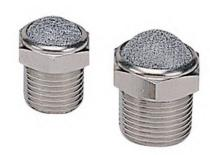
SBN-Series breather vent combines low profile and high air flow into a reality, suitable for many applications, particularly where space is limited. Special screen filiter is fromed by stainless steel wire, offers very high mechanical resistance, guaranteeing long life even under high pressure. Nickel plated brass fitting offers additional corrosion resistance.
