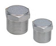
SSBV-Series low profile breather vents are constructed with 300-Series stainless steel materials, they are resistant to atmospheric corrosion, foodstuffs, sterilizing solutions, many organic dhemicals, dyestuffs and wide variety of inorganic chemicals.
