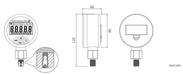
Pressure port equipped with snubber can avoid damage caused by sudden pressure surge of water or oil, improve product durability. When snubber is clogged with contaminants, please use a flat head screwdriver to remove the snubber, clean and reinstall.
